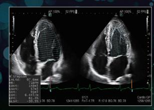
Simpson measurement, which utilizes Al technology\*, automatically recognizes LV, LA and RA intima and measures the volume. Additionally, a wide range of functions are supported to improve the workflow of cardiovascular measurement, such as Doppler Cursor Assist.
